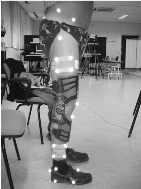
Fig. 3 Anterior and lateral views of the right knee show a MOS Genu ® knee brace with affixed markers.
