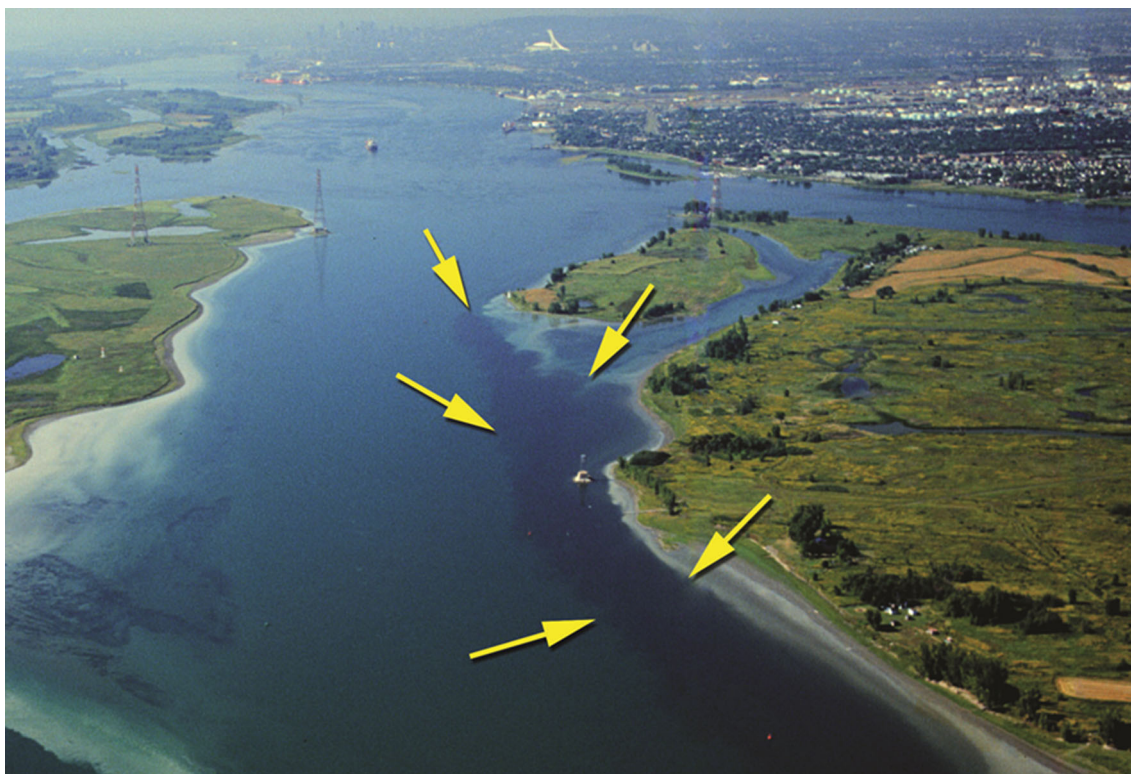
Fig. 2 Aerial photograph of discharge of the Montreal wastewater treatment plant in the St. Lawrence River. Arrows indicate the sewage effluent, which appear as dark blue color. Photograph by Christiane Hudon
