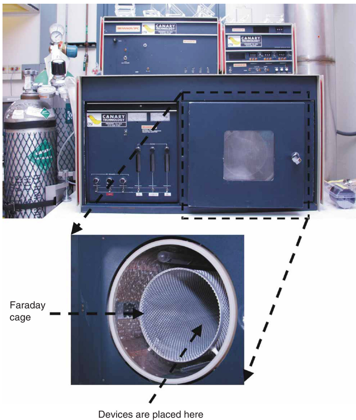
Figure 11. Oxygen plasma device. The Faraday cage (insert) sits inside the vacuum chamber. The device requires the plasma chamber to be evacuated of air and replaced with pure oxygen. The devices sit inside the cage.
