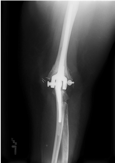
Fig. 4 Axle failure and disassociation of a Coonrad-Morrey implant is evident in this radiograph.
