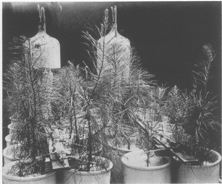
FIG. 2. Drip-cultures at the end of 14 months. Capacity of each carboy is 18 liters. Uniform rate of drip is maintained by means of bottles that serve as constant-level reservoirs. Solution reaches individual cultures by dripping from capillary tubes. For series on left, nitrogen was supplied as calcium nitrate; for series on right, as ammonium sulphate.
