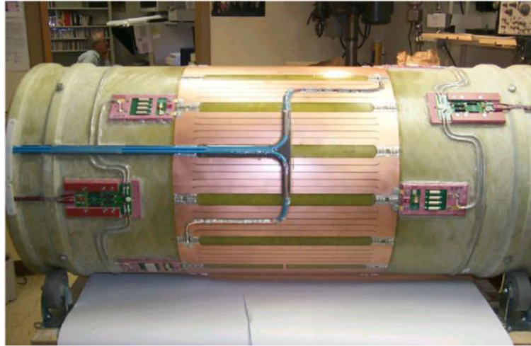
Figure 1. A prototype 3 Tesla Body Coil. Image courtesy of Stanford University Department of Radiology
