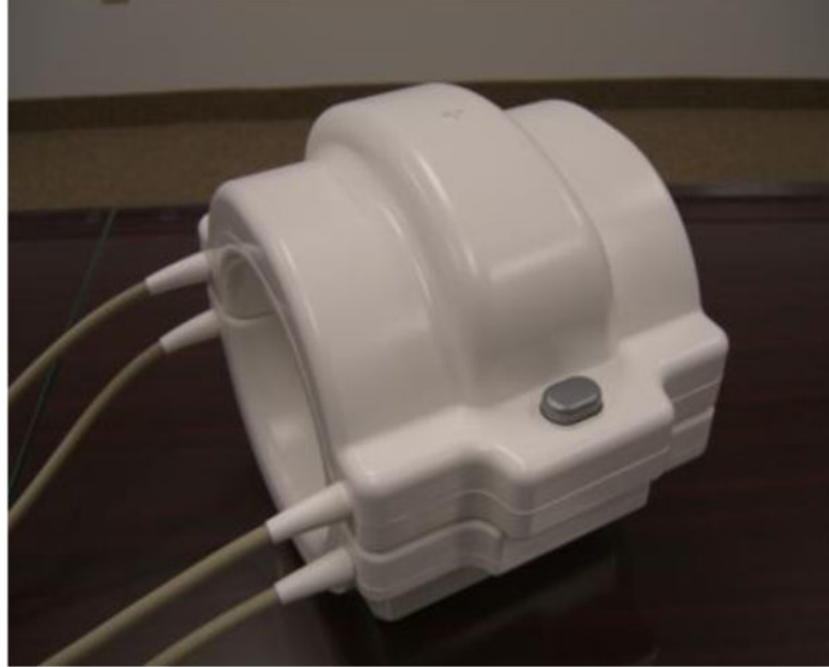
Figure 2. QED 28-Channel Knee Coil (Courtesy of Quality Electrodynamics, OH, USA; Ravinder Regatte, NYU Langone Medical Center, NY, USA; Siegfried Trattnig, the Medical University of Vienna, Vienna, Austria)
