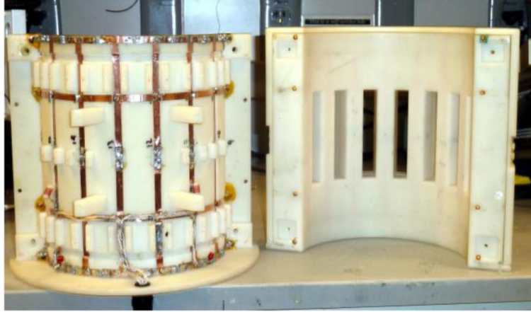
Figure 7. Split 4-ring dual-tuned 1\text{H}/^{23}\text{Na} birdcage knee coil. Image courtesy of Stanford University Department of Radiology.
