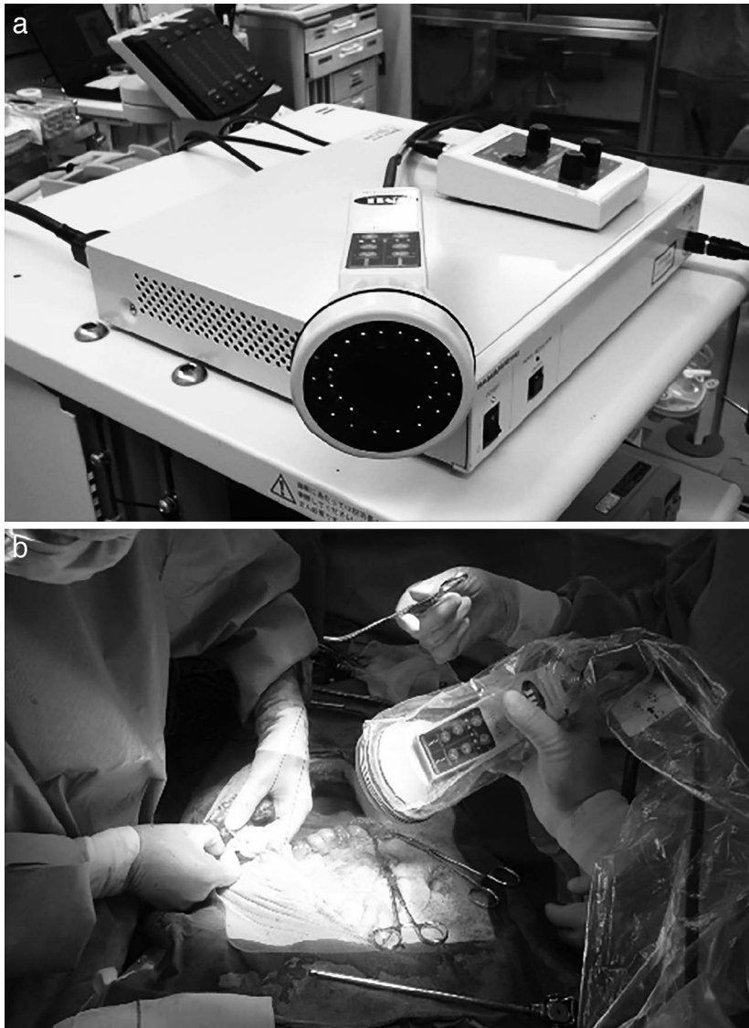
Fig. 1 (a) The PDE system consists of a desktop computer and a CDC camera connected with a flexible line. The light handy-type instrument is very convenient for performing highly sensitive intraoperative observation. (b) This hand-piece instrument allows free observation of the abdominal cavity with high sensitivity.
