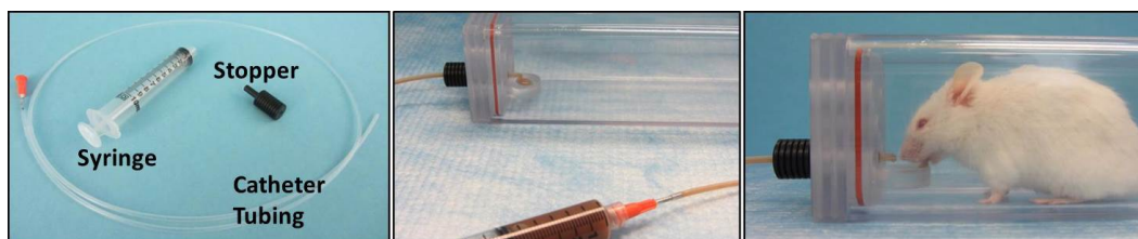
Figure 4: Syringe Delivery System. Left: unassembled components. Middle: assembled components. Right: mouse drinking from peg-bowl in observation chamber. Please click here to view a larger version of this figure.
