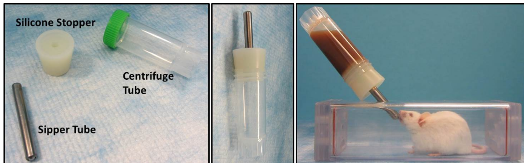
Figure 3: Sipper Tube Bottles. Left: unassembled components. Middle: assembled components. Right: mouse drinking from sipper tube in observation chamber. Please click here to view a larger version of this figure.
