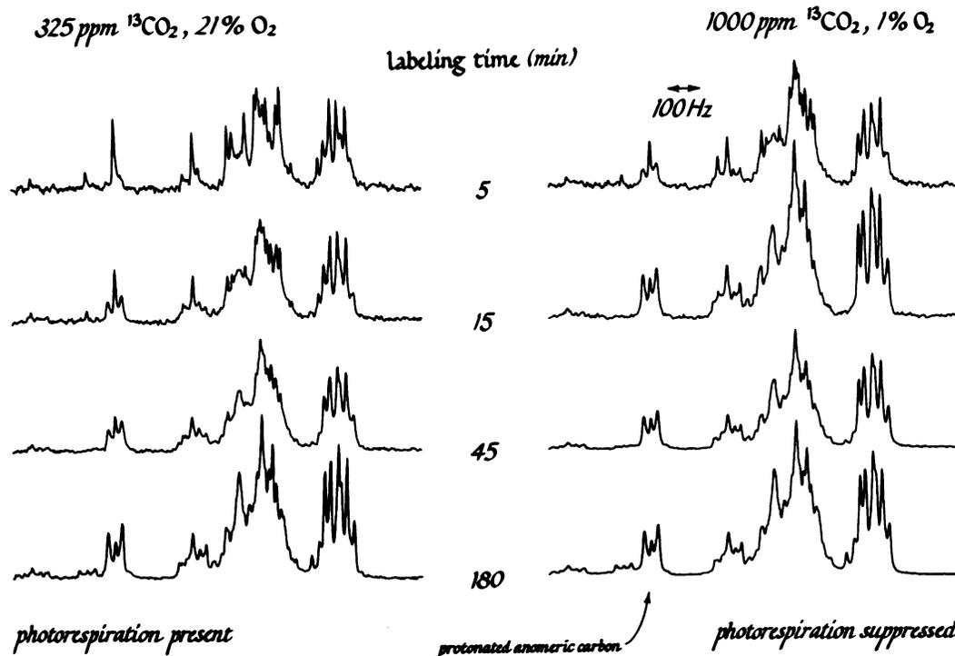
FIG. 2.  $^{13}\text{C}$  NMR spectra of sucrose extracted from soybean leaves labeled with  $^{13}\text{CO}_2$  for 5–180 min using two different gas compositions.
