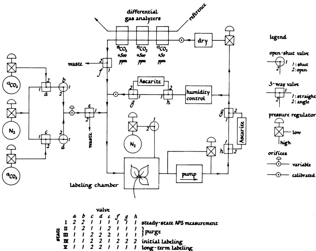
FIG. 1. Gas flow diagram of the <sup>13</sup>CO<sub>2</sub>-labeling system.
