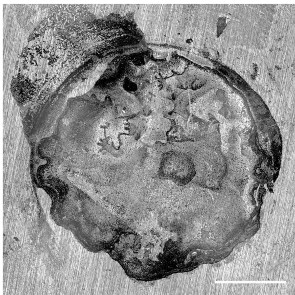
Figure 2 Example of a cohesive failure mode of Biodentine on dentine after 14 d. Original magnification x5. Bar represents 1 mm.
