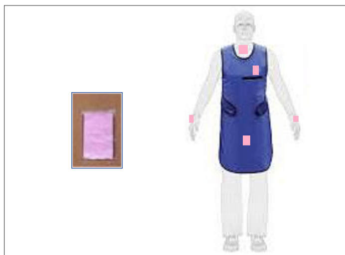
[Table/Fig-1]: TLD Badges used were obtained from Bhaba Atomic Research Centre [Table/Fig-2]: Positioning of the TLD Badges
