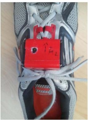
**Figure 1**Foot-mounted accelerometer (Gold Standard) attached to the runner's shoe
