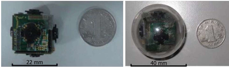
Figure 8 Spherical capsule endoscopy with multiple cameras.
