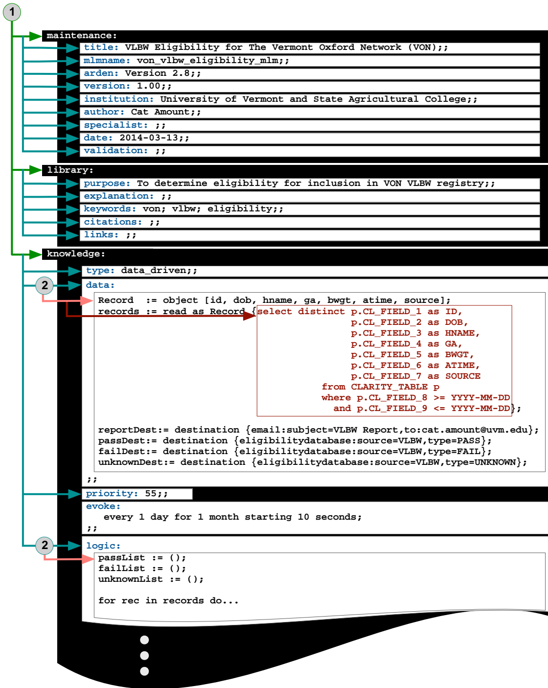
Figure 3: MLM Parsing. A system was developed that (1) used an ANTLR parser generator to identify the MLM categories (maintenance, library, and knowledge) and their contained slots; and (2) used an additional ANTLR parser generator to process the slots and leveraged the Akiban SQL Parser to process SQL statements embedded within the data slot. For this feasibility study, a SQL statement was used to retrieve data from the FAHC EHR reporting database that was used for eligibility determination (ID = Patient identifier; DOB = patient date of birth; HNAME = hospital name; GA = gestational age; BWGT = birth weight; ATIME = admission time; and SOURCE = admission source) according to the criteria depicted in Figure 1.
