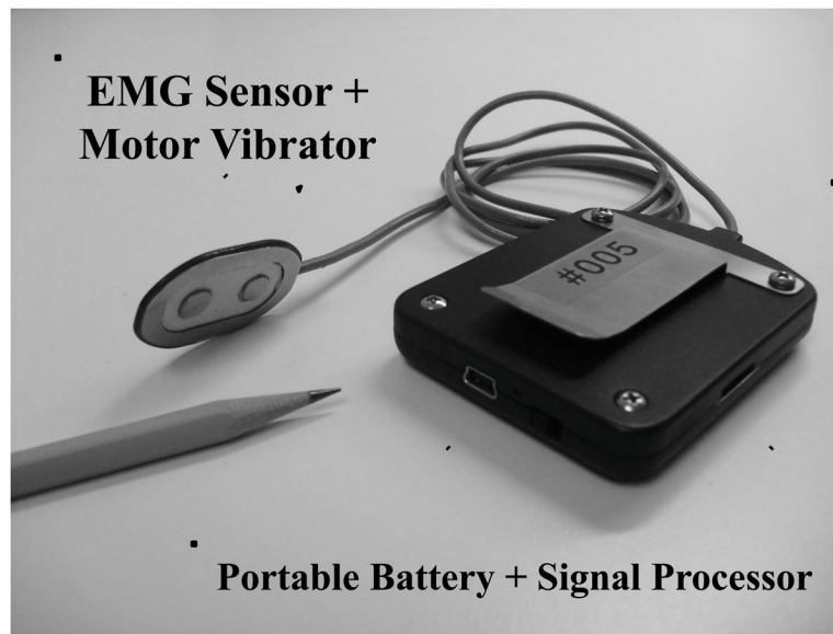
Figure 1. EMG-based biofeedback device with vibration motor embedded. The device alerts the person of his/her muscle activity with smooth changes in the speed of a silent vibration motor. Proportional tactile feedback is achieved by driving the motor with a signal proportional to the estimated EMG power, and the vibration is provided at the site of the active muscle.
