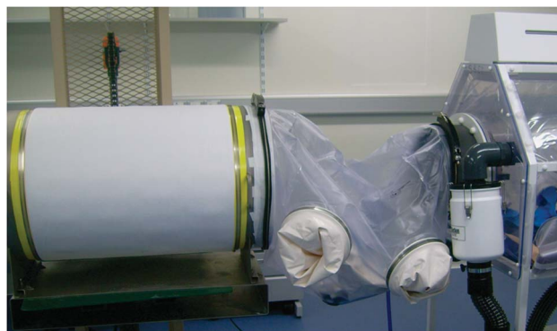
Figure 2 Sterile connection between a material drum and a flexible film isolator. The large steel drum contains sterile materials to be imported into the isolator, such as food, bedding, or cages. The drum is sealed and autoclaved and then connected to the isolator via a plastic sleeve that is sterilised by spraying with 2% peracetic acid, which then permits transfer of the sterile material into the isolator.
