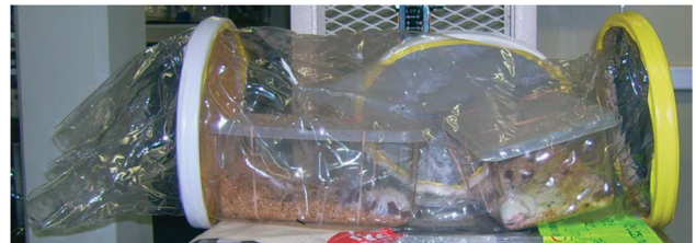
Figure 4 Specialised transport sleeve. The photo shows an example of a specialised transport sleeve developed to allow shipping of germ-free animals between facilities. The example shown is available from Taconic. Many germ-free facilities have developed their own transport devices that reflect the design of their isolators. Such transport containers allow importation of germ-free or isobiotic mice into isolators at the new facility and ensure hygiene is maintained during transport.
