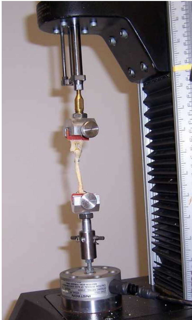
Figure 2. Mechanical Testing Setup with all-inside suture repair. Sandpaper was affixed with cyanoacrylate to the distal 3 millimeters of the distal phalanx and to the proximal 10 millimeters of the tendon stump. Pressure clamps were used to secure the proximal end of the tendon and the distal end of the distal phalanx.
