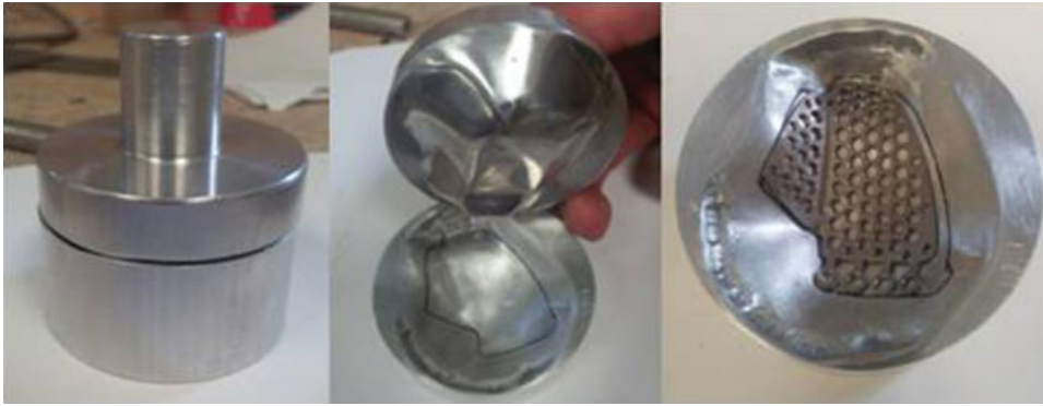
Fig. 4 An orbital implant press to mold the implant to desired anatomical contours. A separate left and right press exists in our department.
