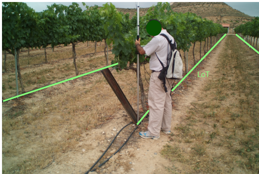
Figure 6. Process of measuring the line of trunks (LoT) with RTK-GPS.
