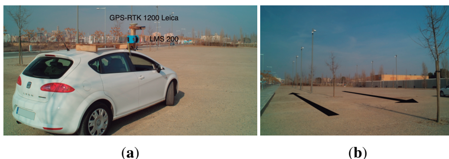
Figure 15. Setup of test: test for checking the perpendicularity of the scanning plane. (a) LiDAR mounted on a car; (b) test zone showing car paths.
