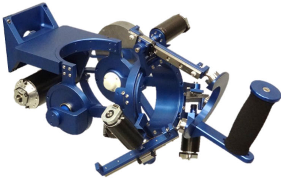
Figure 1. MAHI Exo-II, A 5-DOF Powered Exoskeleton
