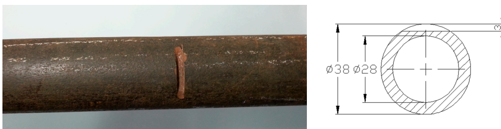
Figure 4. The photo and the schematic diagram of the notch.
