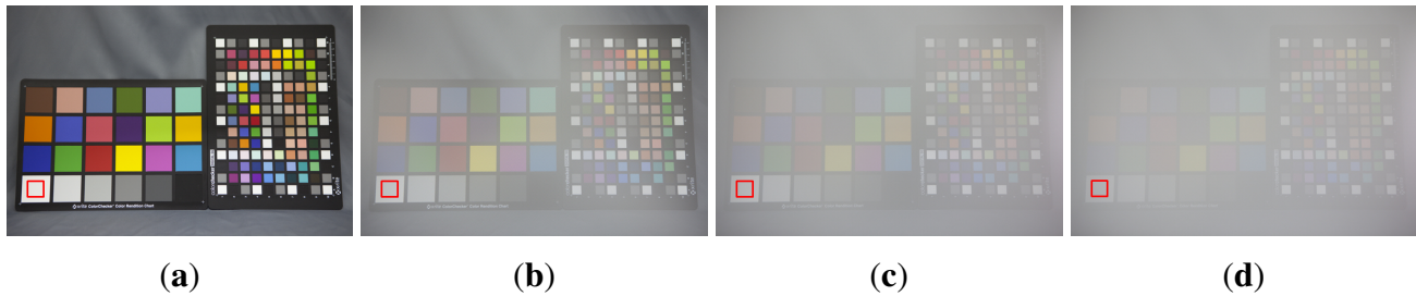
Figure 1. Test images acquired from the same indoor scene with a different amount of steam generated by a humidifier: (a) the haze-free image without steam; and (b–d) the hazy images with different amounts of steam.
