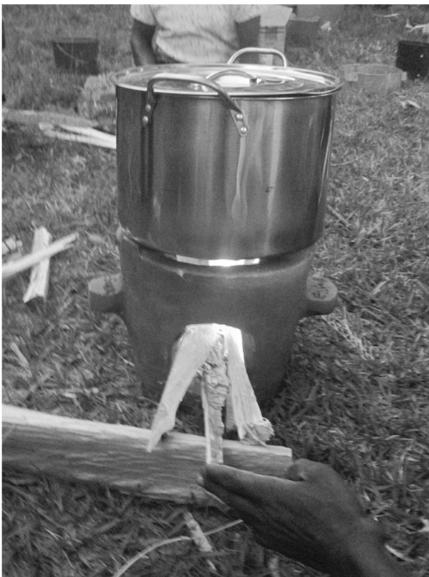
Figure 1 The Chitetezo stove is a simple clay cookstove for burning solid fuels that aims to reduce exposure to household air pollution by burning fuel more efficiently than an open fire, thereby reducing fuel consumption and producing fewer waste combustion products.
