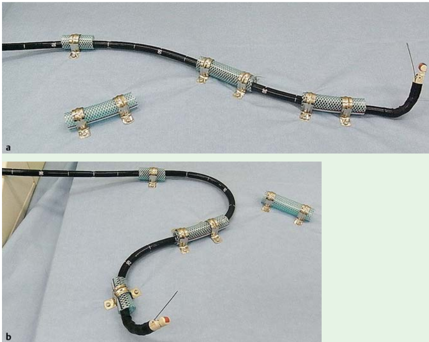
Fig. 1 Bench simulator: a straight therapeutic scope position; b curved scope position.
