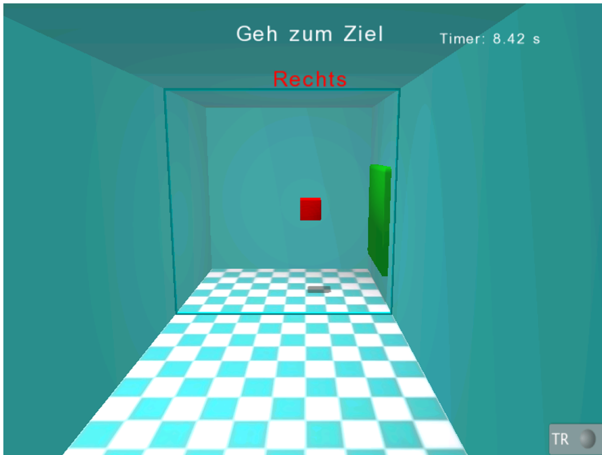
Fig 2. Visual representation of the WORKSPACE assessment package. Screenshot of the WORKSPACE assessment. A room was presented on the screen. The patient looked directly into this room. The end effector of the robot (the position of the patient's hand) was represented as a small red cube. In the shown situation the patient had to move to the green target position to the right.
