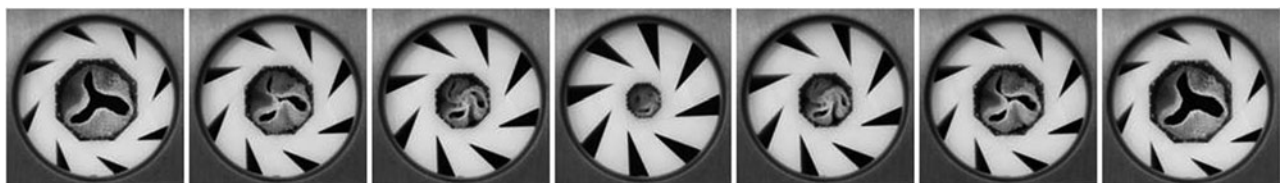
FIG. 3. Crimping of the tube-in-stent valve. The diameter was decreased from 22 mm to 8 mm and the valves were kept in the crimped state for 20 min before letting it return to the original size.
