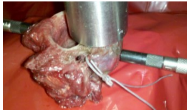
Fig. 3. Experimental Set-up for Intact Cervical Spine. The anterior sensor measures anterior bulge, the posterior sensor tracks the displacement of the bone movement.
