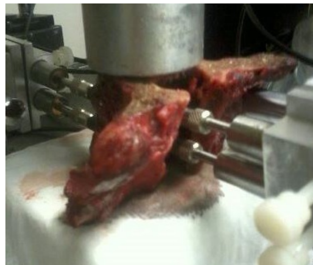
Fig. 4. Experimental Set-up for Cervical Spine Post Laminectomy, the additional sensor is added to measure the posterior bulge.
