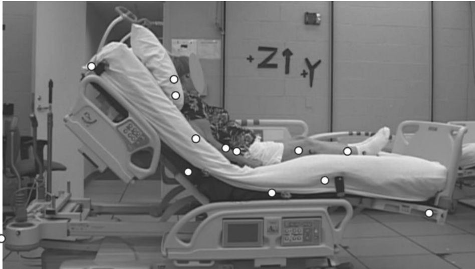
Figure. Motion marker positions for a participant positioned on the bed including 7 markers on the body and 6 markers on the bed. Reprinted with permission from Kermit Davis. Copyright November 10, 2014, Kermit Davis, University of Cincinnati, Cincinnati, Ohio.
