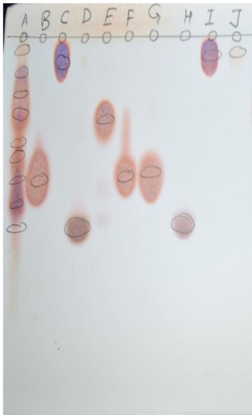
Fig. 1 The Schematic representation of the amino acids (TLC plate) of the mushroom with standards a) Agaricus bisporus b) Methionine c) Arginine d) Tryptophan e) Threonine f) Valine g) Isoleucine h) Phenylalanine i) Lysine j) Histidine
