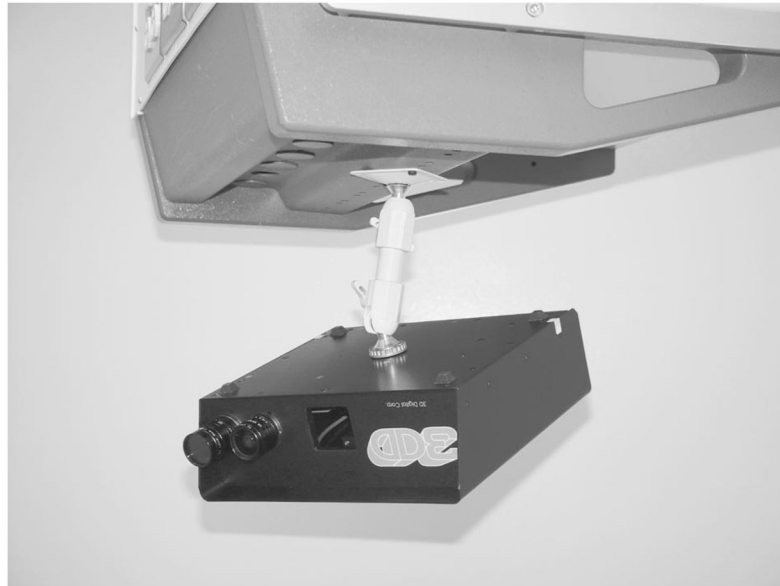
Fig. 1. The RealScan 3-D Laser range scanner mounted to an OR mechanical arm.
