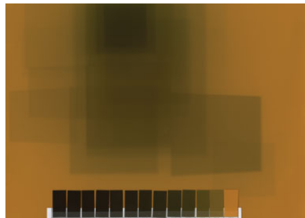
Fig. 1 Radiochromic film (14 inches \times 17 inches) from a fenestrated and branched endovascular repair showing the two-dimensional radiation dose distribution. Film darkness is correlative to increased radiation dose.
