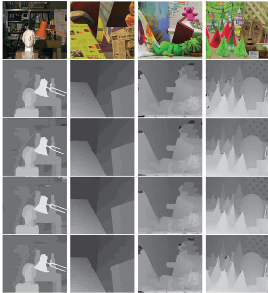
Figure 9. Experimental results of the Middlebury data sets. The 1 st row: the reference images; The 2 nd row: the disparity maps established with ST2. The 3 rd row: the disparity maps established with Cross_Sp+WMF. The 4 th row: the disparity maps established with GF. The 5 th row: the disparity maps established with MST.
