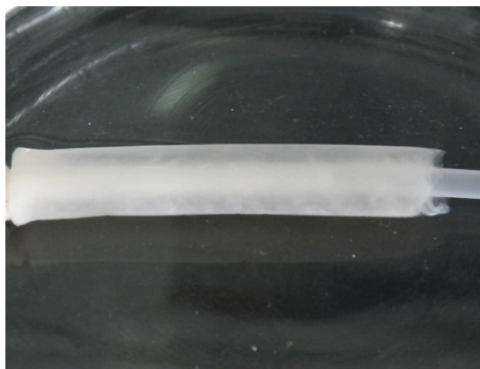
FIGURE 4: Photo of tubular BNC material produced in the double-silicone-tube bioreactor inoculated with Kombucha.
