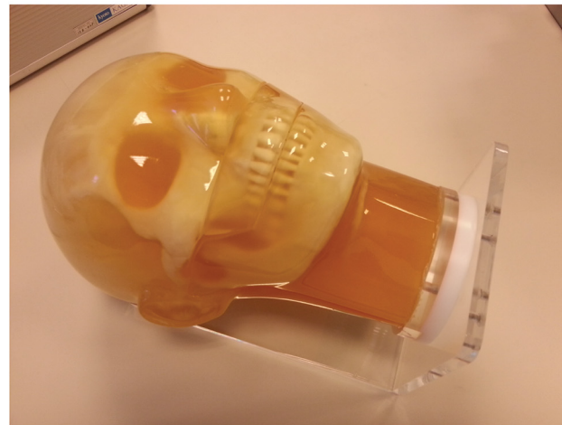
Fig 1. The Kyoto Kagaku PH-47 head/neck phantom. (a) The assembled phantom. (b) The disassembled jaw.
