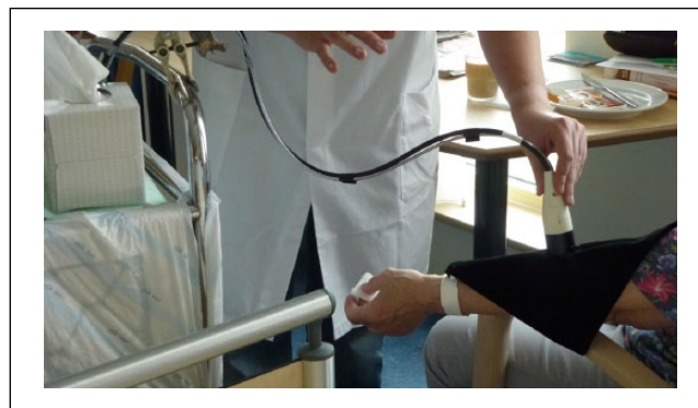
Figure 2. Measurement with the dedicated measurement head; the black cloth prevents stray light from entering the probe, and stray laser emission.
