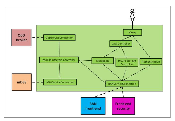
Figure 1. Internal structure of the smartphone user interface.
