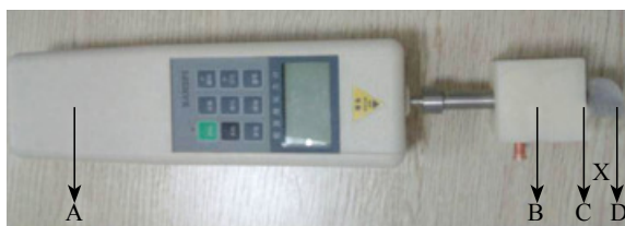
Figure 1. The device used for the abdominal wall tension (AWT) measurements. This instrument can measure the required thrust to produce displacement (mm). A: thrust meter; B: self-made device; D: oval head. Vertical pressure during the measurement drives the device to the abdominal wall and stops when C is touched by the abdominal wall. X is the vertical displacement of the abdominal wall sag. The thrust is recorded by A. AWT is defined as thrust/displacement (N/mm).
