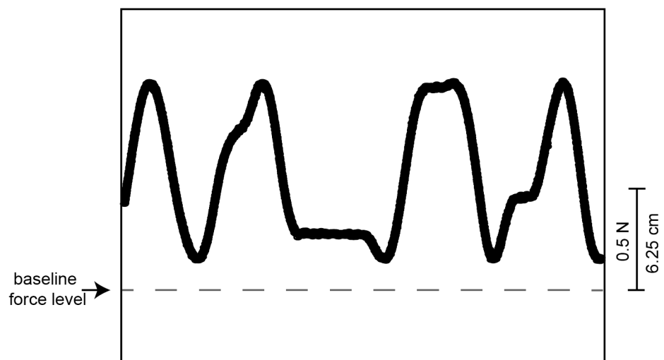
Fig 1. Image of the complex waveform used in the CIVTT. Subjects were instructed to produce a time-varying abduction force by pressing on a small force transducer using their index finger in order to track the complex waveform. The application of force onto the transducer drove an oscillographic display in which the cursor moved automatically from left to right at a rate of 5.9 cm/sec.
