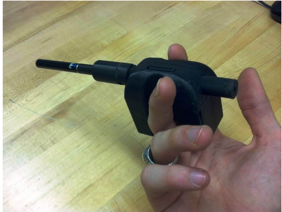
Fig 1. RIT wireless Personal Use Monitor (wPUM). The RIT wPUM is employed to record subject's use of electronic cigarettes in their natural environment.
