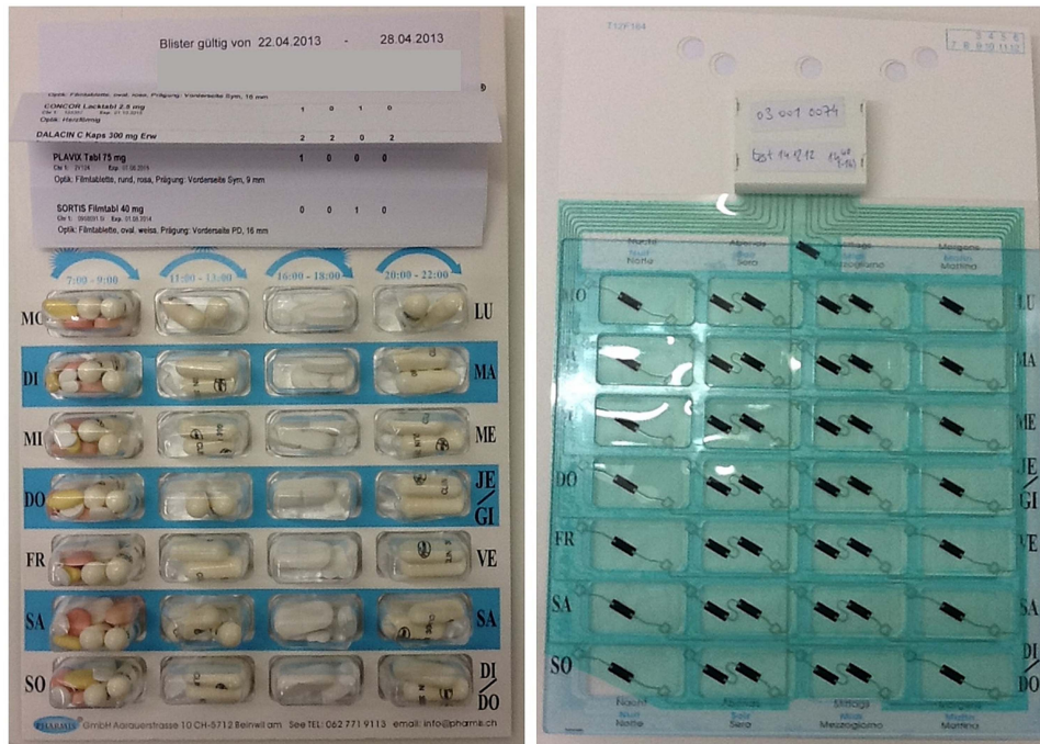
Figure 1 Electronic multidrug punch card front (left) and back with affixed Polymedication Electronic Monitoring System (POEMS; right).
