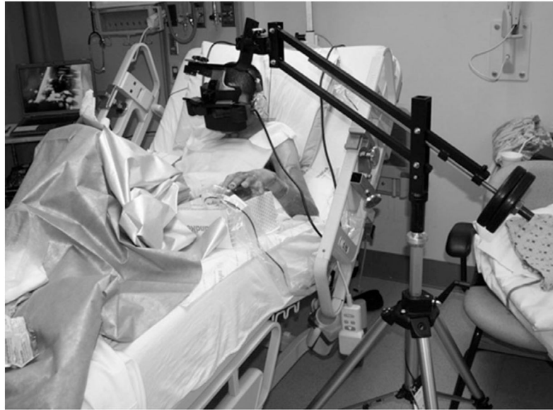
Figure 1. US Army soldier receiving immersive virtual reality (VR) to reduce his pain during severe burn wound care. The unique robot-like arm mounted VR goggles designed by Hoffman and built by Jeff Magula at the University of Washington, Seattle, holds the VR goggles near the patient's eyes weightlessly, reducing the amount of surface contact (if any) needed with the patient. Photo and copyright Hunter Hoffman.
