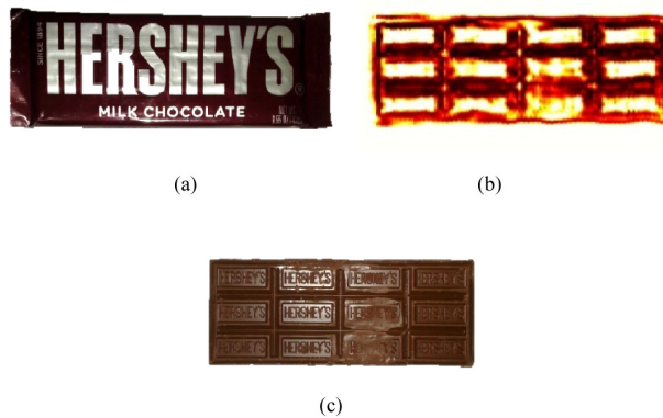
Fig. 9. (a) Digital photograph of a wrapped chocolate product (packaging material: polyethylene (PE)). (b) Clipped image from a continuous-wave (CW) sub-THz transmission image by the polygonal mirror scanning method, where the intensity legend was skipped for better comparison with its visible image. (c) Digital photograph of the chocolate (138 mm \times 50 mm \times 5 mm) after removing the wrapper, where some parts of the chocolate are melted.
