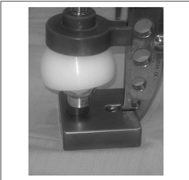
Figure 2 The special device used to lock the head into the liner. Note the head placed under the polyethylene liner. On tightening this device with a screw mechanism, the liner is pushed down and on to the head. The inner diameter of the liner is smaller than the head diameter, which means that once locked in, the head cannot come out.
