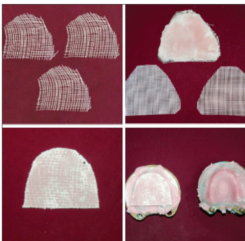
Figure 6: Reinforcement using glass fiber and polyethylene prepreg.
