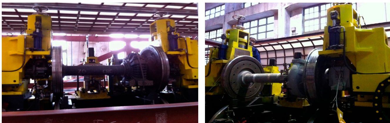
Figure 2. Railway axle bearing test-rig.
