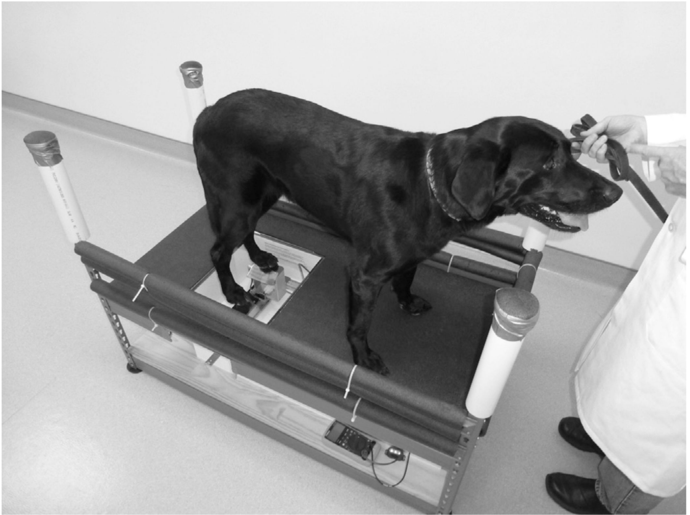
Fig. 1. Dog shown standing on the Canine Thermal Escape System (CTES). This was a client-owned dog that had not seen the CTES previously. The CTES used for thermal quantitative sensory testing (QST) is housed in a purpose made wooden box. This is incorporated into a heavy-duty metal shelving system with the metal struts covered in protective foam. Dogs stand on the top surface, which is covered in rubber matting except for the area of glass that covers the area containing the halogen bulb. During testing, one individual is positioned in front of the dog or to the left side, gently dissuading the dog from moving. The other individual is kneeling on the floor, operating the arm connected to the carriage head with the halogen light source in it and positioning it under the paw. Positioning was facilitated by observing the reflection in the mirror attached to the carriage head.
