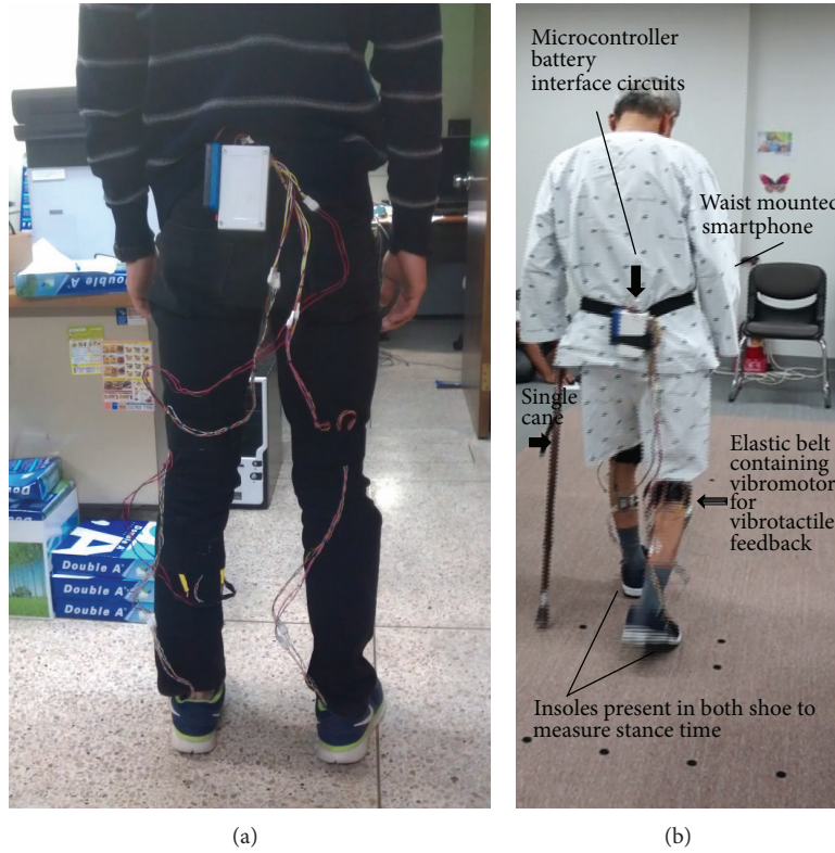
FIGURE 3: Device attachment: (a) healthy young subject and (b) individual with stroke.
