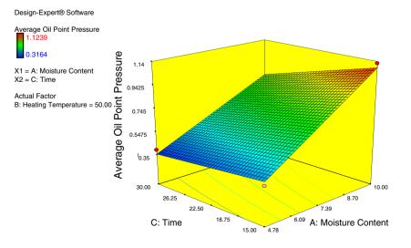
**Fig. 4** Response surfaceof oil point pressure of moringa oleifera seed with heating temperature and time at the moisture content of 6.00 %
