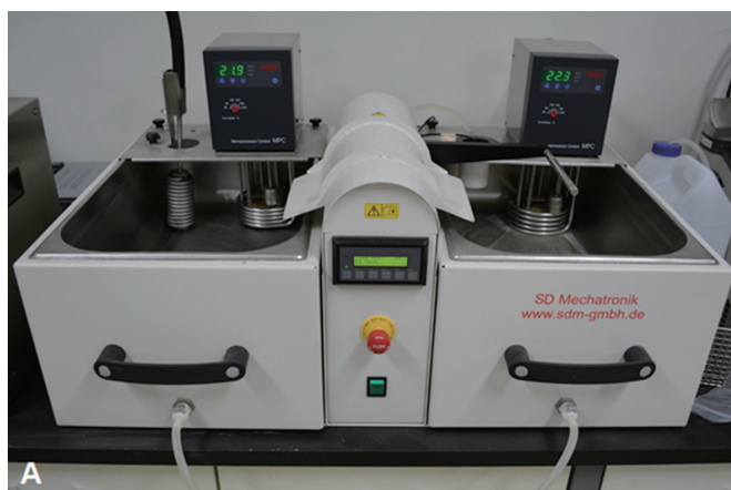
Fig. 2. Artificial aging apparatus: (A) thermocycling apparatus, (B) chewing simulator.
