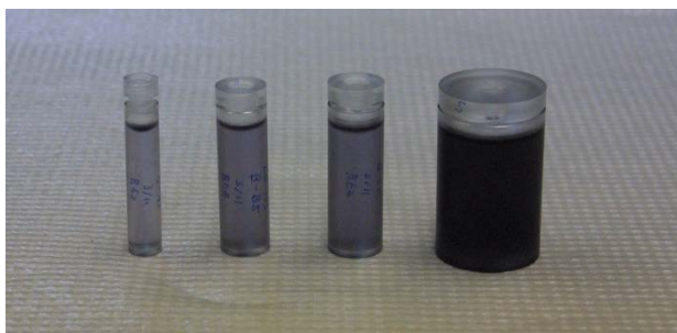
Fig. 1. Photograph of a set of ^{133}\text{Ba} epoxy sources prepared for and calibrated in this study. The sources appear dark due to a dye that was added to the epoxy during manufacturing as a visual indicator of uniform mixing.
